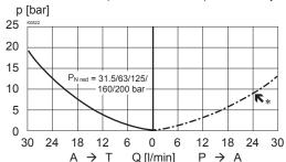
$\Delta p = f(Q)$  Pressure loss/flow characteristics over non-return valve
