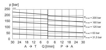
p<sub>red</sub> = f (n) Pressure adjustment characteristics [at Q = 0 l/min (static)]
