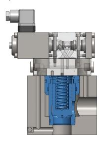
Installation and control of a slip-in cartridge valve
